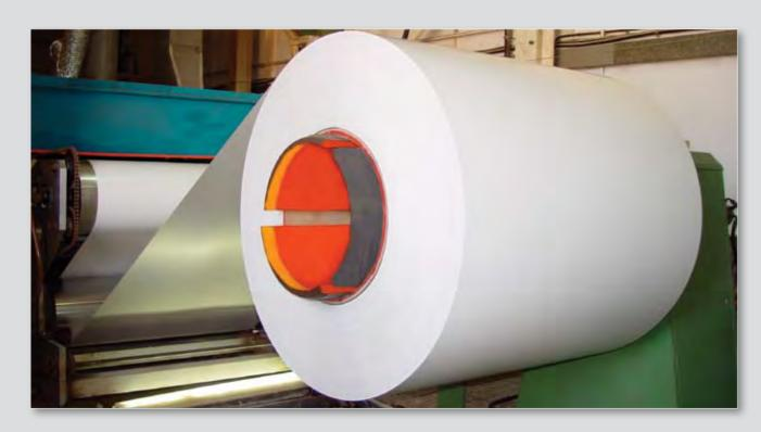
CoilCoat is a highly efficient coating plant that coats aluminum, galvanized and aluzinc coils. Three coating lines exist within the Group that coat and laminate polyester, PVDF and Plastisol with embossed textures. Harwal Group uses innovative coil coating production methods and processes that generate consistent production runs. CoilCoat caters to many leading manufacturers of roofing, cladding, composite panels, ceilings, window blinds, sporting goods and appliances.
